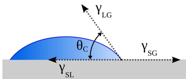
Figure 2: Contact Angle
